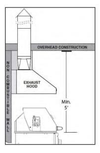
**Combustible Overhead Construction:** Exhaust hood required.
