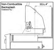
Clearance between grill and protected combustible wall (i.e. a non-combustible wall in front of a combustible wall to serve as a barrier. This can be accomplished by brick or a metal stud finished with non-combustible substrate. Clearance Fig. 2). The grill must have a minimum of 14" right, left and rear clearance from the protected combustible wall. (The 4" non-combustible material clearance, plus an additional 10" clearance between the grill and protected wall.)
