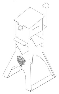
4. Bolt the fryer to the stand using 4 of the  $\frac{1}{20}x \frac{3}{4}$ " bolts.
