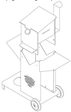
7. Secure the fryer to the cart with 4 of the  $\frac{4}{20}$  x  $\frac{3}{4}$  bolts through the slots in the front and back.
