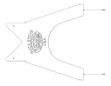
3. Turn the bolted stand upright and you can use the 4 bolts you just put in, to level it on your surface. With the help of a second person pick up the fryer and place it on the stand pieces, with the stand cradling the fryer.
