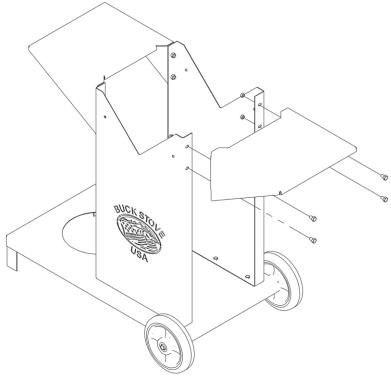
6. With the help of a second person pick up the fryer and place it on the stand pieces. With the upright cradling the fryer on the inside.
