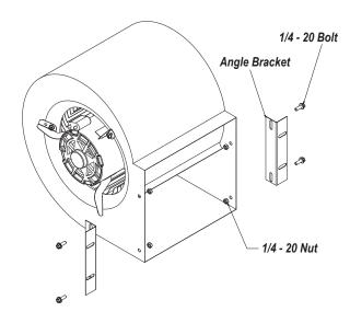
2. Line up the blower with the pre-drilled holes on the backside of the furnace and firmly attach with the screws provided.
