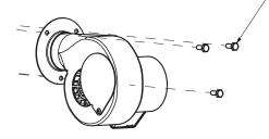
6. To install the fan limit control, remove cover, attach with three (3) #8 screws in predrilled holes and replace cover.
