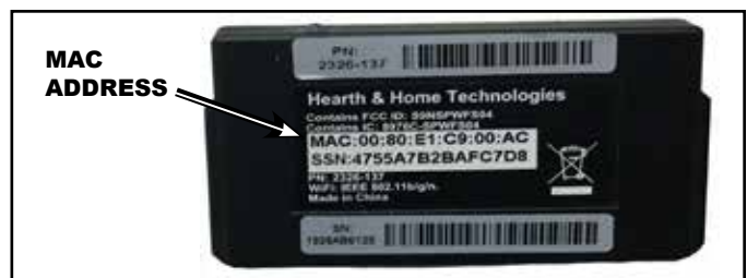
Figure 1 Wi-Fi module MAC Address Location
