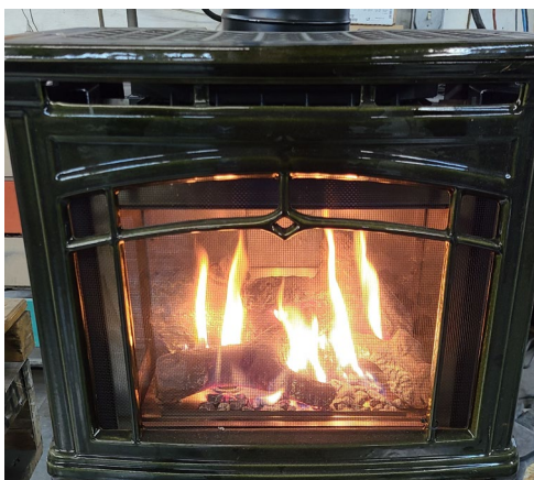
Figure 31 - Typical Burner Flame Appearance
